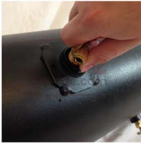
Thread in your 1/2"x1/4" fitting into both ports on the front of your air tank.
