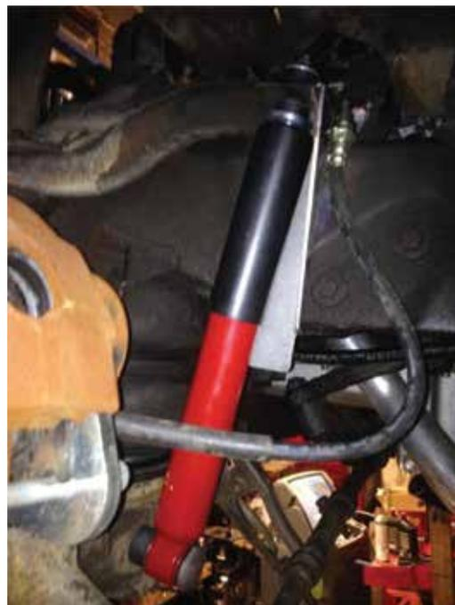
Slide the upper tower over the top of the shock stud. Let it fall into place on the frame and mock up where your relocater bracket will be welded. Tack it in place and test the shock for no binding / clearance issues - using a floor jack can help.
