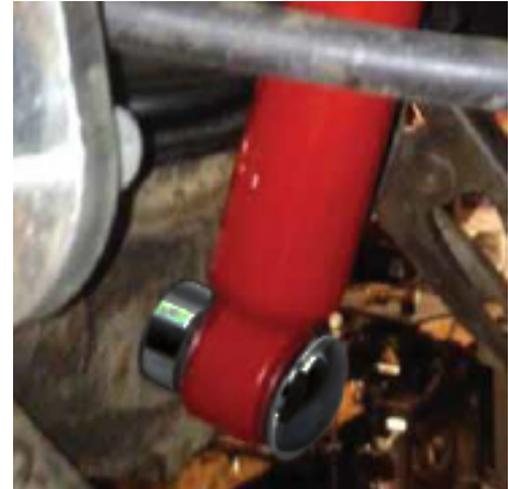
With air out of bags, fully compress the A Arm. Hold up one compressed shock and one fully extended to mock up where your hole and shock tower will land. Make sure you have clearance and no binding issues then drill a hole for the shock stud.
